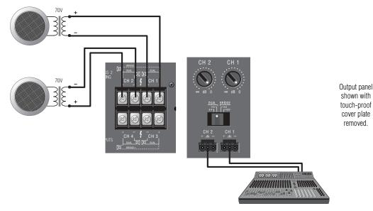
Figure 3.7 System Wiring and Control Settings, Dual Mode, 70V.
